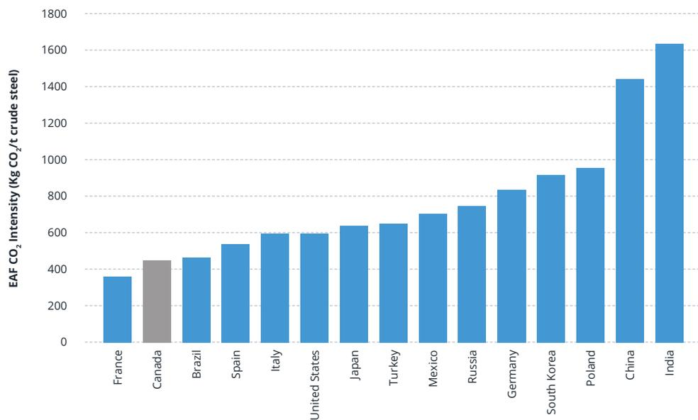
Figure 2: Carbon intensity of EAF steel production (2016)<sup>36</sup>
